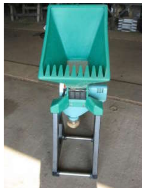
Canola-kit attached to the minibatt. The grains are fed into the thresher through the hopper.
